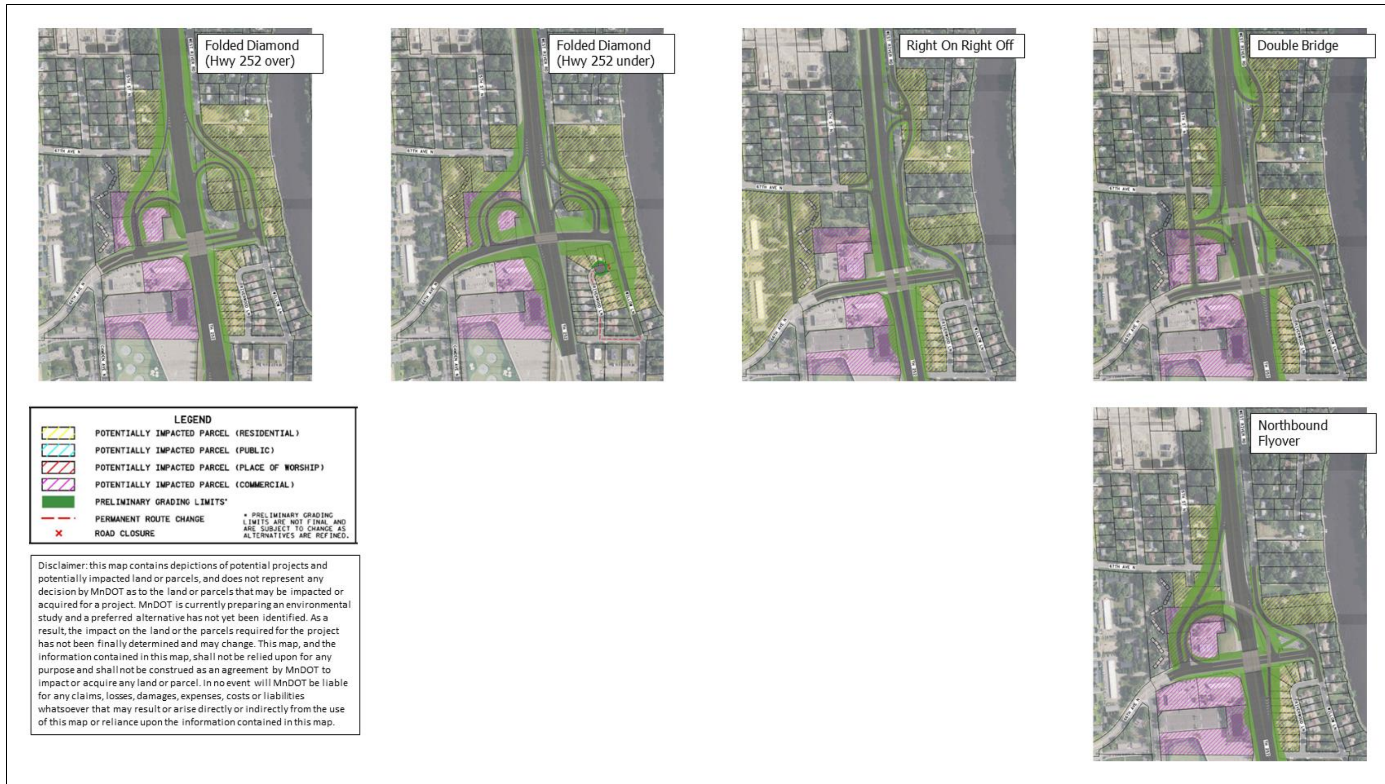
Figure 7.41 Hwy 252 and 66 th Avenue Interchange Concepts
