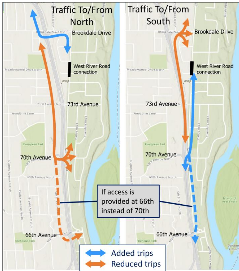
Figure 7.32 Hwy 252 and West River Road Reconnection
