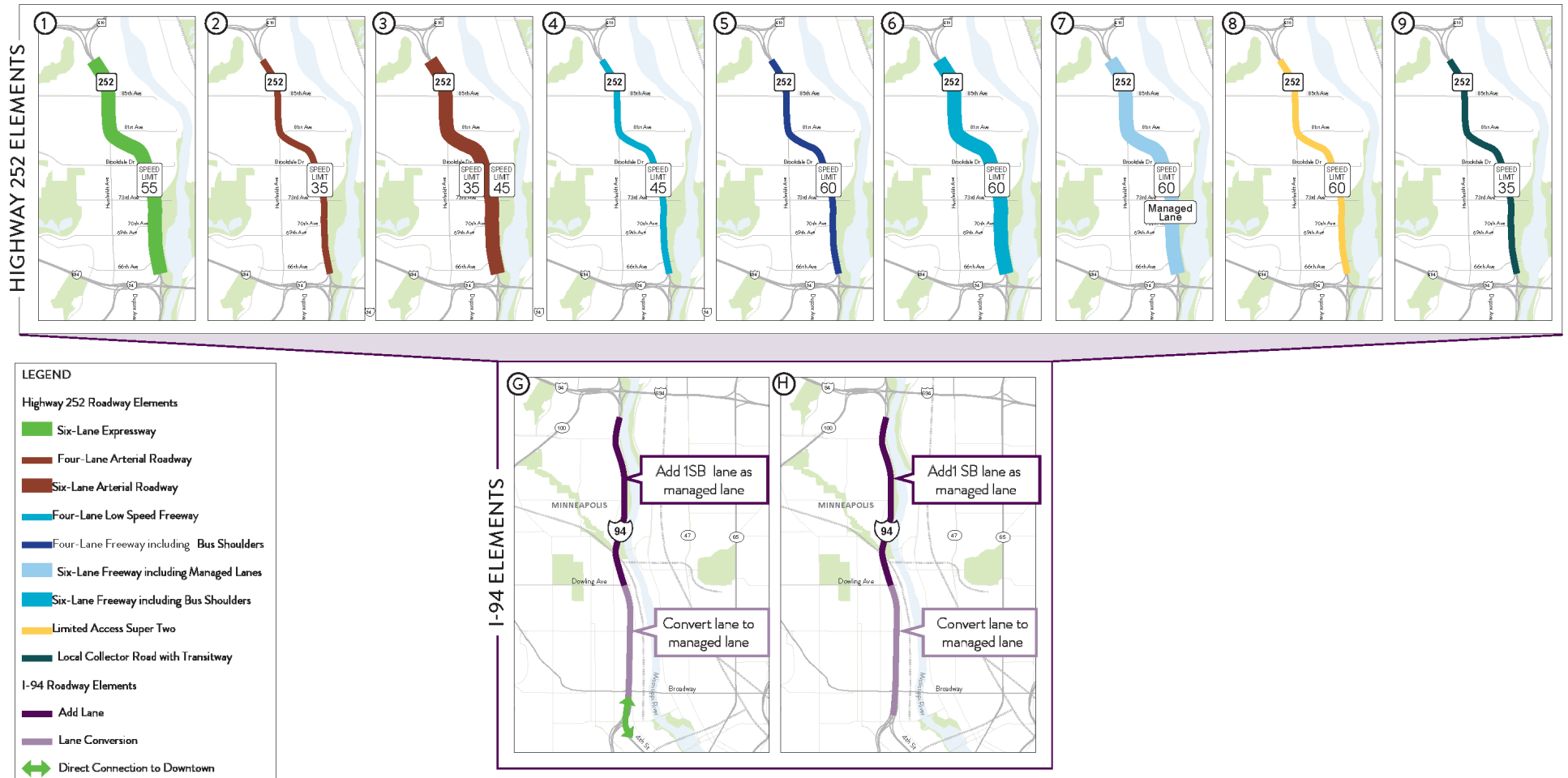
Figure 7.18 Hwy 252 and I-94 Corridor Alternatives Package 4
